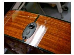
Tail End Smash Cracking on the tail end of the guitar. It can range from a small crack on the binding seam to multiple cracks through the wood that shatter the finish.
