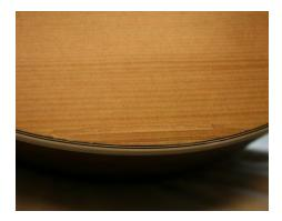
**Top Compression** Buckling in the top caused by impact to the side of the guitar.
